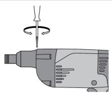
Insert the tip of a screwdriver between the protective sleeve and the power tool.
