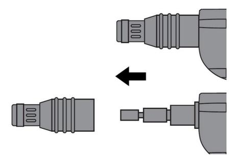
• Pull the depth gauge forward, away from the power tool.
