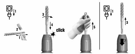
Fit the accessory tool or, respectively, remove it.
