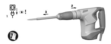
> Pull the accessory tool locking ring back as far as it will go and remove the accessory tool.
